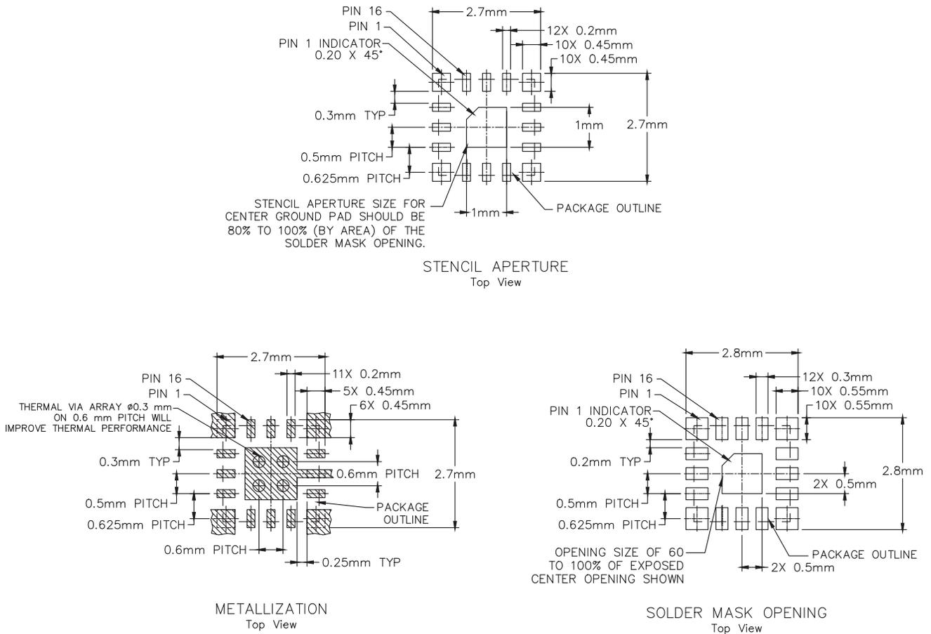
NOTE: THERMAL VIAS SHOULD BE RESIN FILLED AND CAPPED IN ACCORDANCE WITH IPC-4761 TYPE VII VIAS. 30-35UM Cu THICKNESS IS RECOMMENDED.
