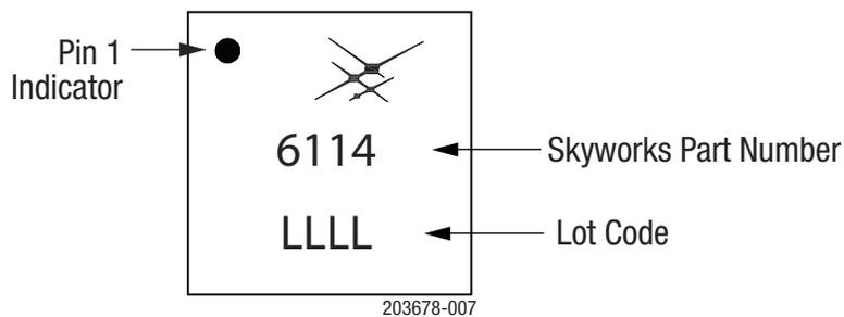
Figure 7. SKY66114-11 Typical Part Marking (Top View)
