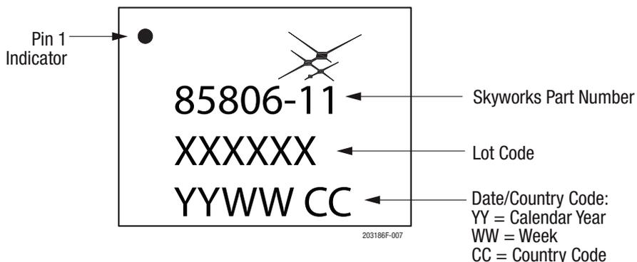
**Figure 7. SKY85806-11 Typical Part Markings (Top View)**
