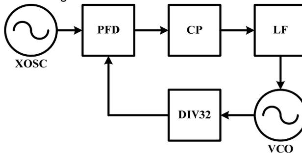
The PLL chain circuit is supplied by internal voltage regulator to ease the PA pulling and crystal spur issue
