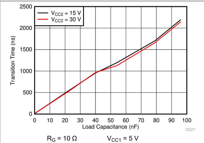
**Figure 7-28.  $t_f$  Fall Time vs Load Capacitance**
