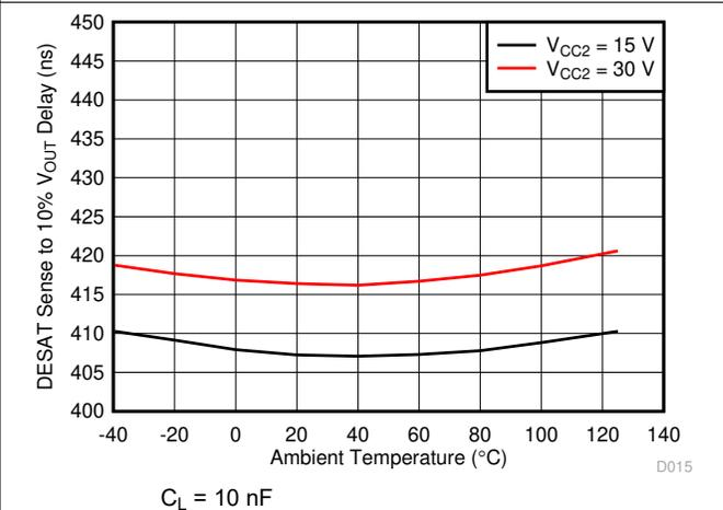
**Figure 7-30. DESAT Sense to  $V_{OUT}$  10% Delay vs Temperature**
