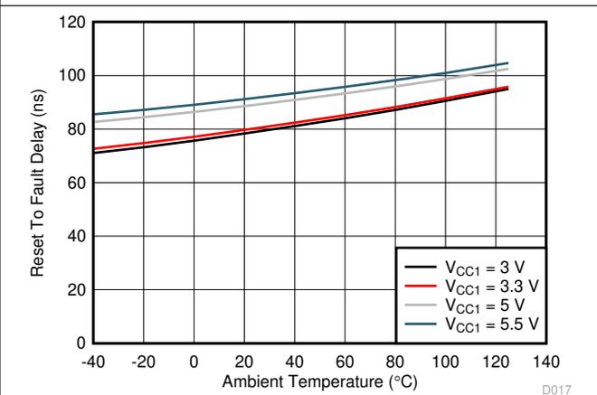
**Figure 7-32. Reset to Fault Delay Across Temperature**
