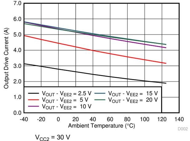
Figure 7-5. Output Low Drive Current vs Temperature
