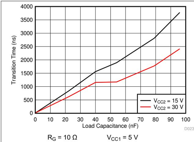
**Figure 7-27.  $t_r$  Rise Time vs Load Capacitance**
