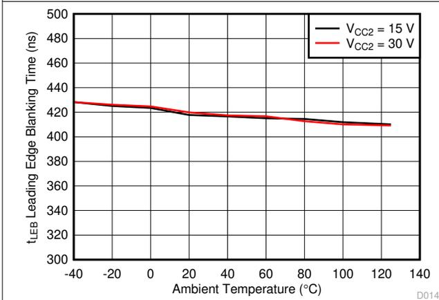
**Figure 7-29. Leading Edge Blanking Time With Temperature**
