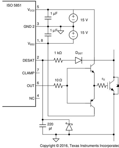
Figure 10-10. Current Buffer for Increased Drive Current
