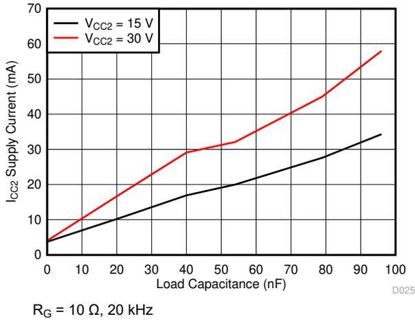
**Figure 7-21.  $I_{CC2}$  Supply Current vs Load Capacitance**
