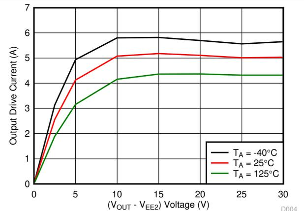
Figure 7-7. Output Low Drive Current vs Output Voltage
