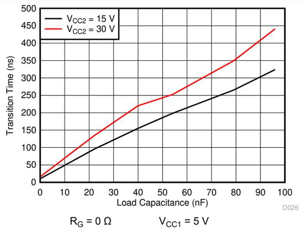
**Figure 7-26.  $t_f$  Fall Time v. Load Capacitance**
