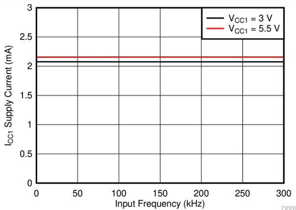
**Figure 7-19.  $I_{CC1}$  Supply Current vs Input Frequency**
