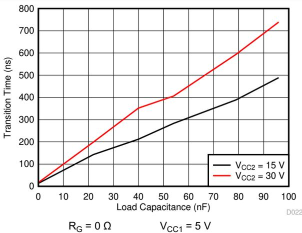
**Figure 7-25.  $t_r$  Rise Time vs Load Capacitance**
