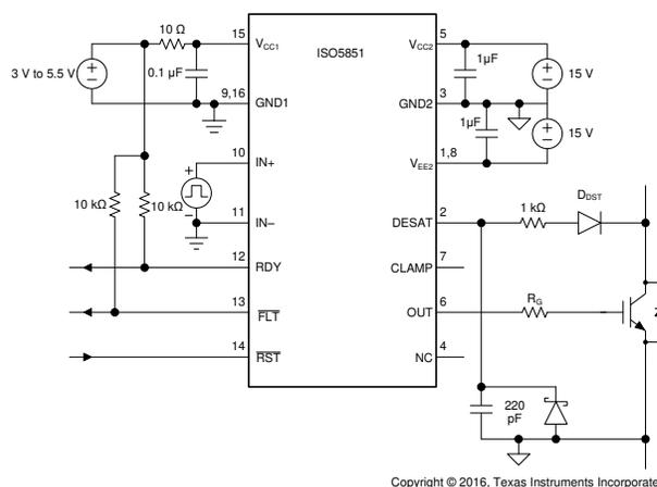
Figure 10-3. Bipolar Output Supply
