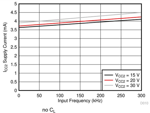
**Figure 7-20.  $I_{CC2}$  Supply Current vs Input Frequency**
