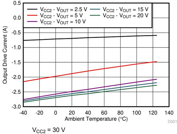
Figure 7-4. Output High Drive Current vs Temperature
