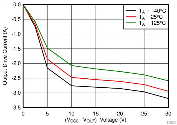
Figure 7-6. Output High Drive Current vs Output Voltage
