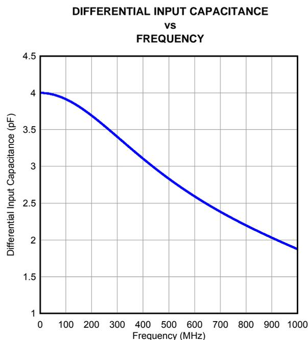
**Figure 53. ADC Analog Input Capacitance ( $C_{in}$ ) Across Frequency**
