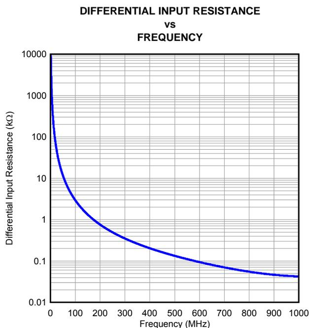
**Figure 52. ADC Analog Input Resistance ( $R_{in}$ ) Across Frequency**
