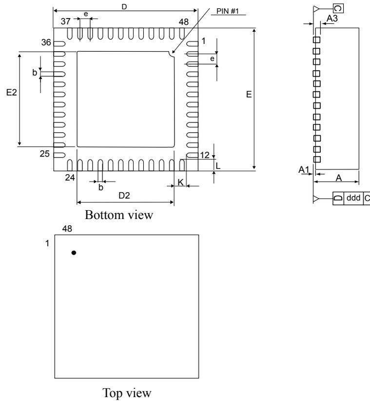
**Table 9. QFN 7X7-48 L package mechanical data**
