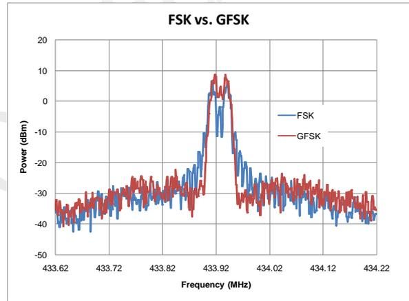
**Figure 6. FSK/GFSK Spectrum,
