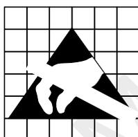
**Caution!** ESD sensitive device. Precaution should be used when handling the device in order to prevent permanent damage.
