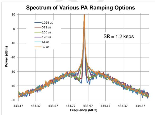
**Figure 7. Spectrum of PA Ramping,
