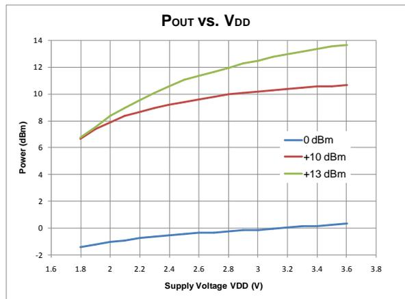
**Figure 8. Output Power vs. Supply
