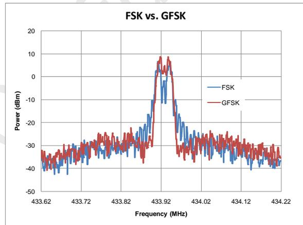
Figure 6. FSK/GFSK Spectrum,
