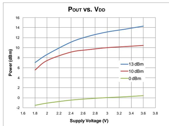
Figure 8. Output Power vs. Supply
