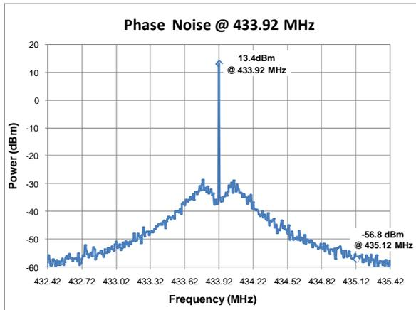
Figure 4. Phase Noise,  $F_{RF} = 433.92$  MHz,
