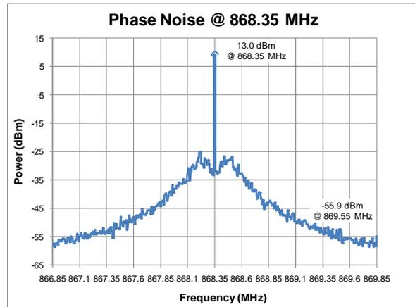
Figure 3. Phase Noise,  $F_{RF} = 868.35$  MHz,
