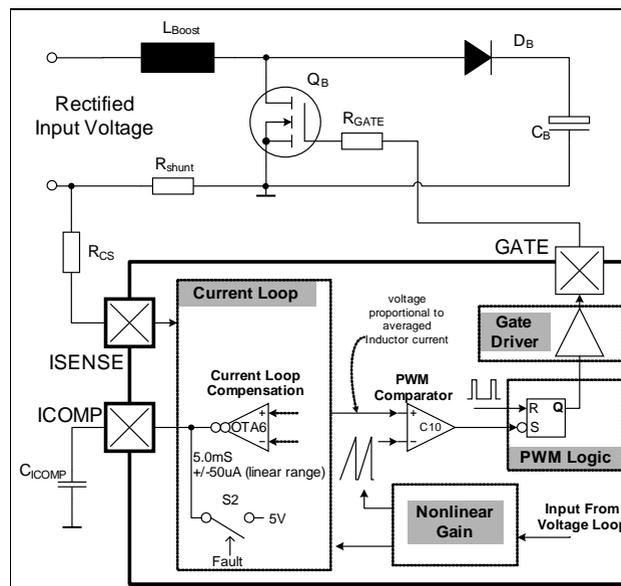
Figure 8 Complete System Current Loop
