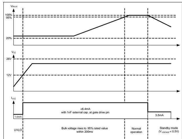
Figure 3 State of Operation respect to VCC
