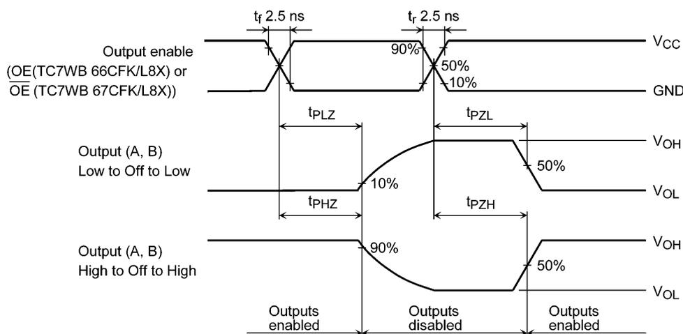
Fig. 11.2.2 AC Waveform  $t_{PLZ}$ ,  $t_{PHZ}$ ,  $t_{PZL}$ ,  $t_{PZH}$
