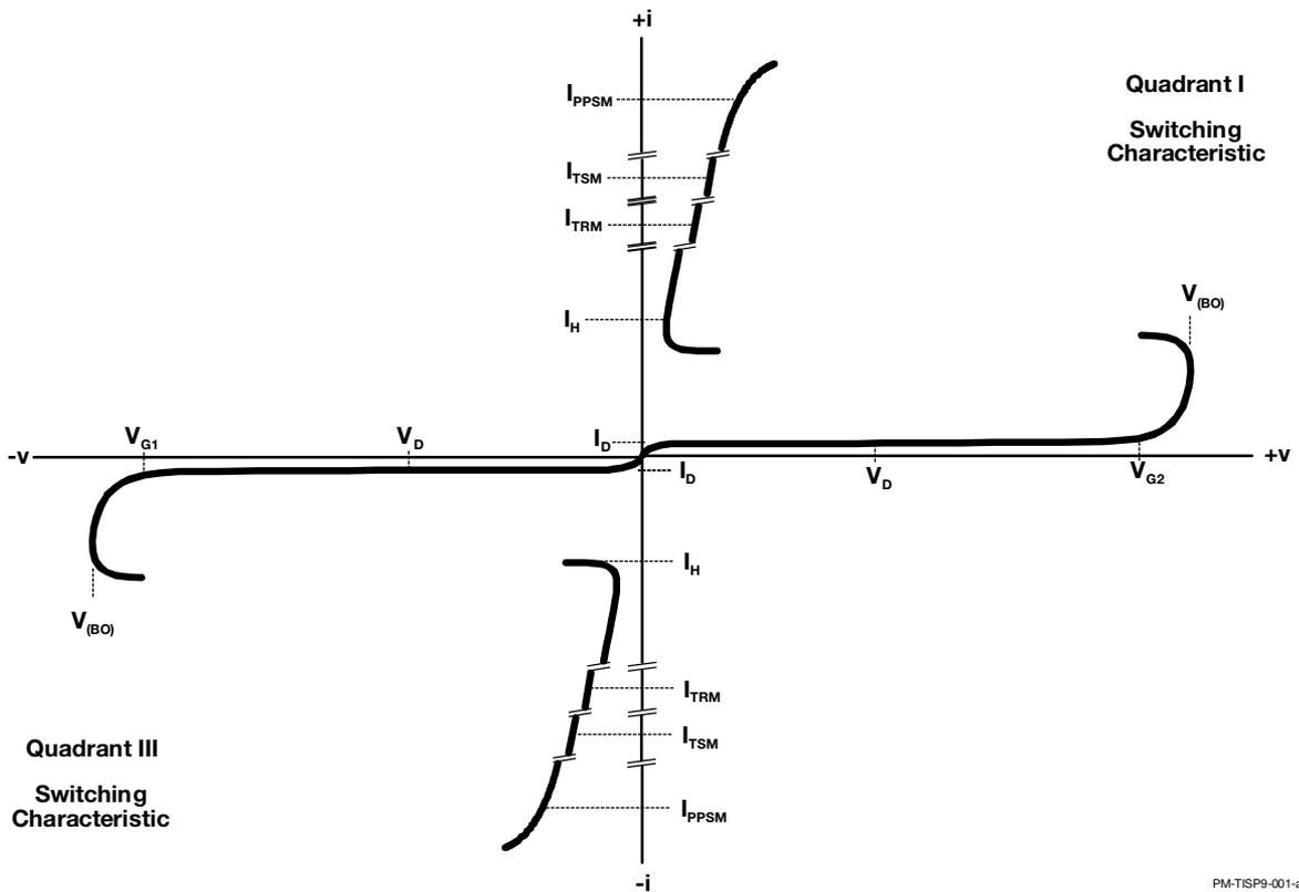
**Figure 1. Voltage-Current Characteristic**
