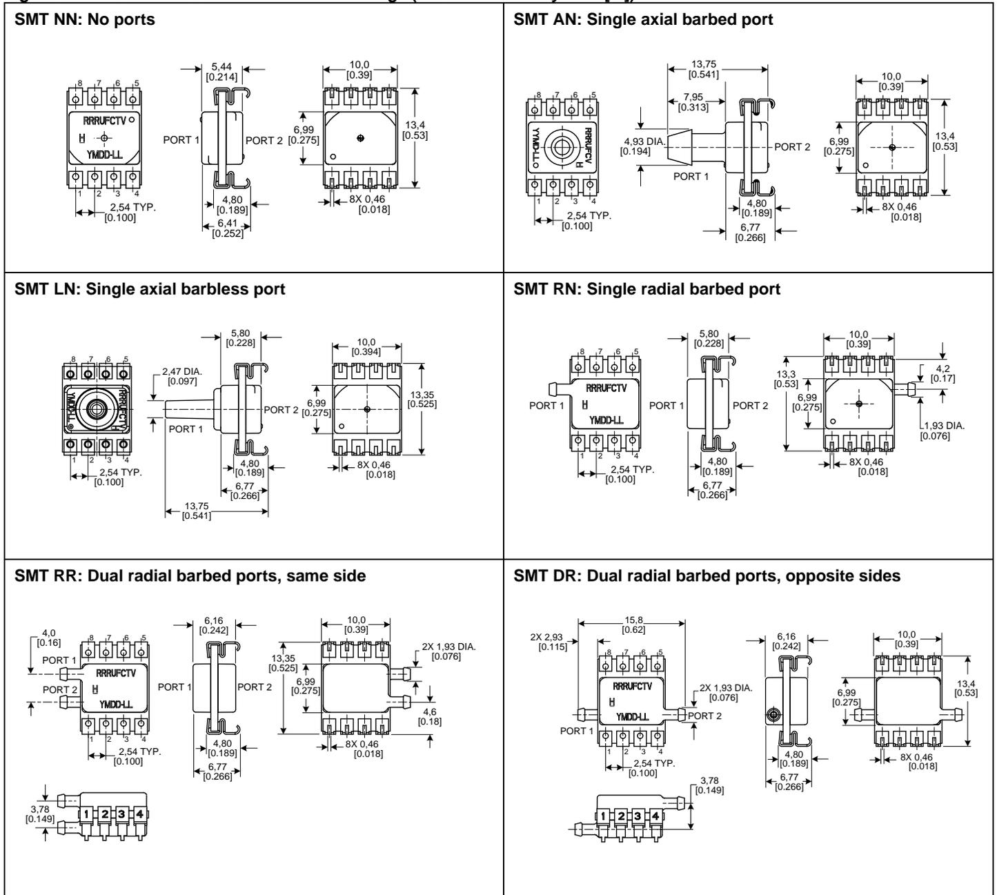
±1% Total Error Band, Digital Output, 1 psi to 150 psi (60 mbar to 10 bar)
