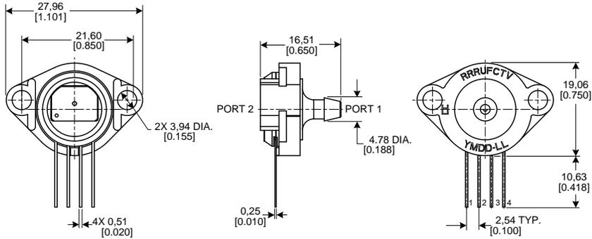
**SIP NB: Fastener mount, dual axial ports, same side**
