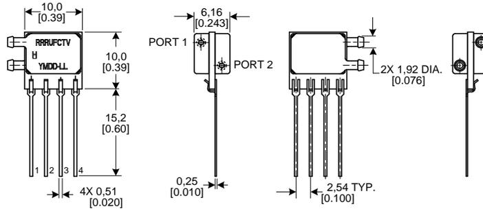
±1% Total Error Band, Digital Output, 1 psi to 150 psi (60 mbar to 10 bar)
