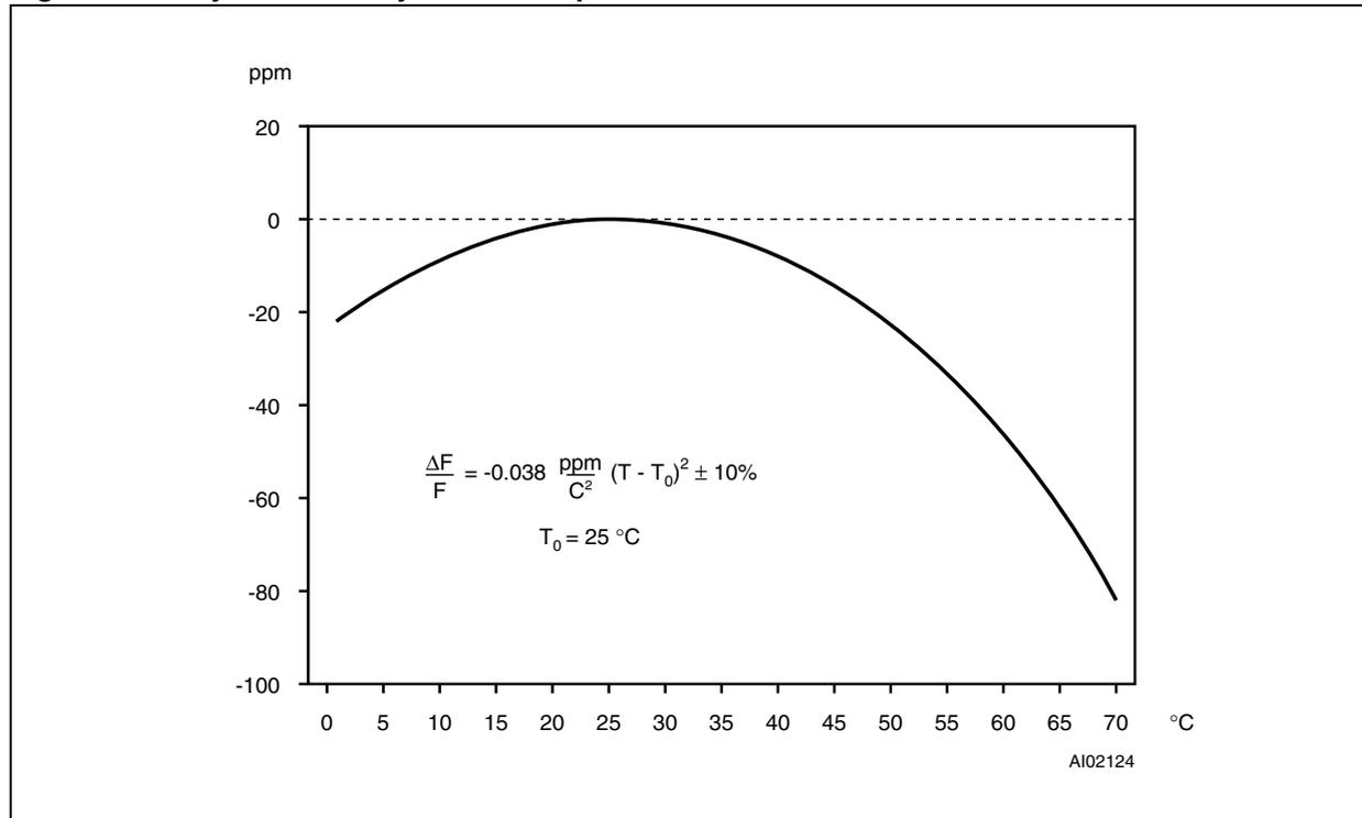
**Figure 9. Clock calibration**
