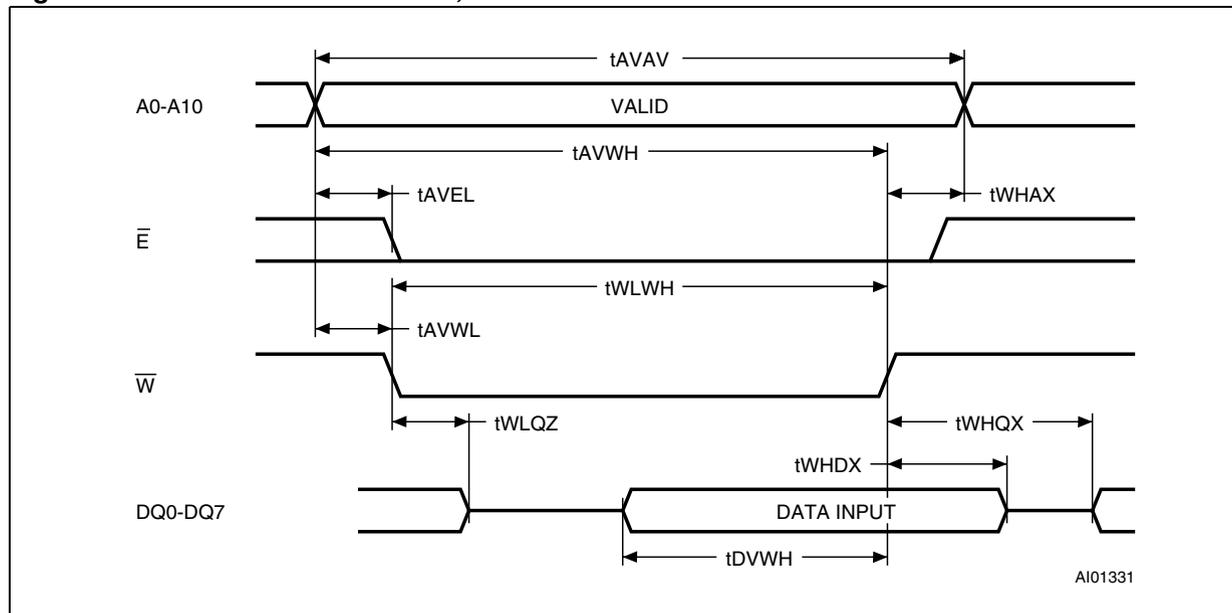
Figure 6. Chip enable controlled, write AC waveforms
