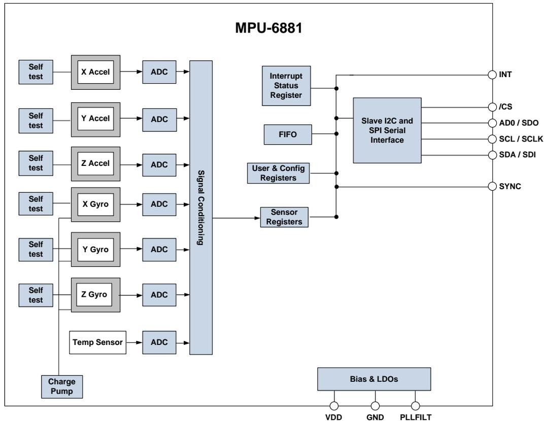
**Figure 5 MPU-6881 Block Diagram**
