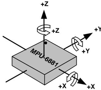
**Figure 13 Orientation of Axes Sensitivity and Polarity of Rotation**
