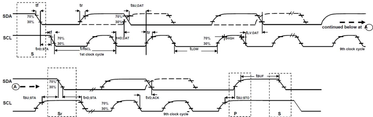
**Figure 1 I<sup>2</sup>C Bus Timing Diagram**
