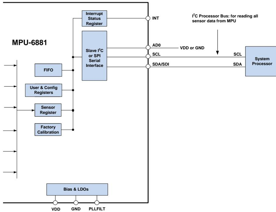
**Figure 6 MPU-6881 Solution Using I2C Interface**
