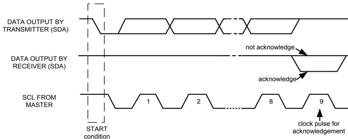
**Figure 9 Acknowledge on the I<sup>2</sup>C Bus**
