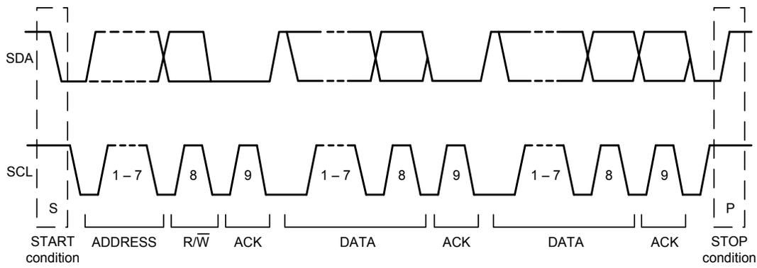
**Figure 10 Complete I<sup>2</sup>C Data Transfer**
