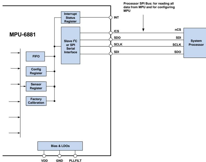
Figure 7 MPU-6881 Solution Using SPI Interface
