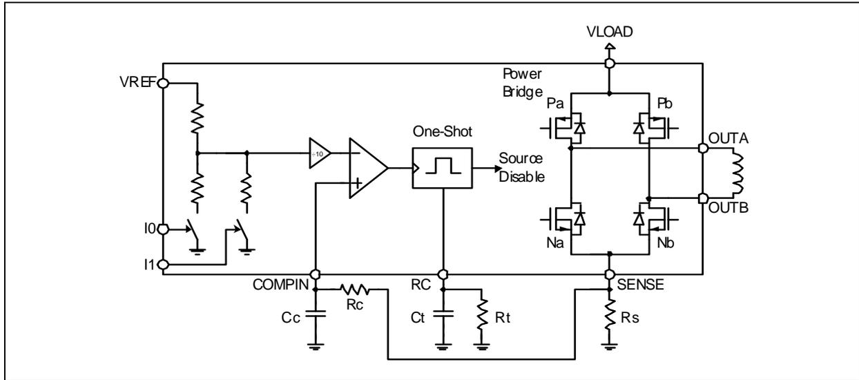
**FIGURE 3-2:** PWM Current Control Circuit Principle (Channel 1 Shown)
