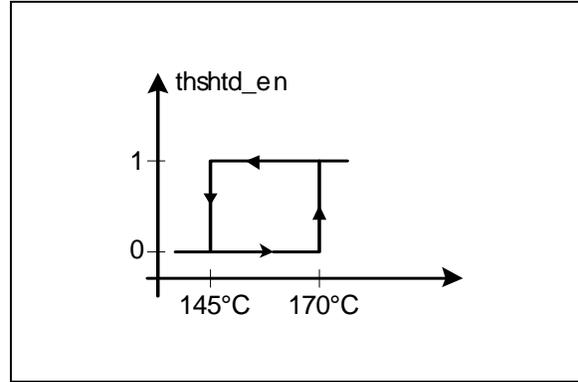
**FIGURE 3-4:** Thermal Shutdown Output vs. Temperature Showing Hysteresis
